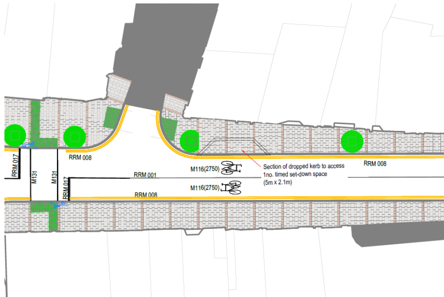
Figure 6.0 -Set down area Lower Castle Street
